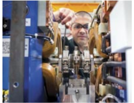
The close spacing of all components in the MBA storage ring requires every design of every fitting to be checked for proper function and proper installation and adjustment. Here, the spacing and fit of vacuum bellows between magnets are being checked on a prototype assembly.
