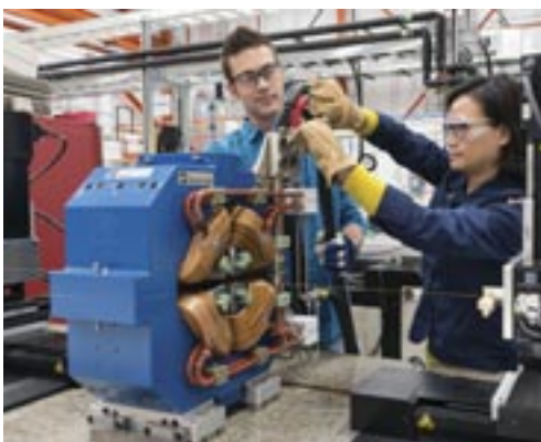
APS-U engineers make adjustments to the first APS-U production-series quadrupole magnet on the magnetic measurement test stand in Bldg. 314. This magnet is the first of 1321 industrially fabricated magnets that will steer the electron beam in the new MBA storage ring.
