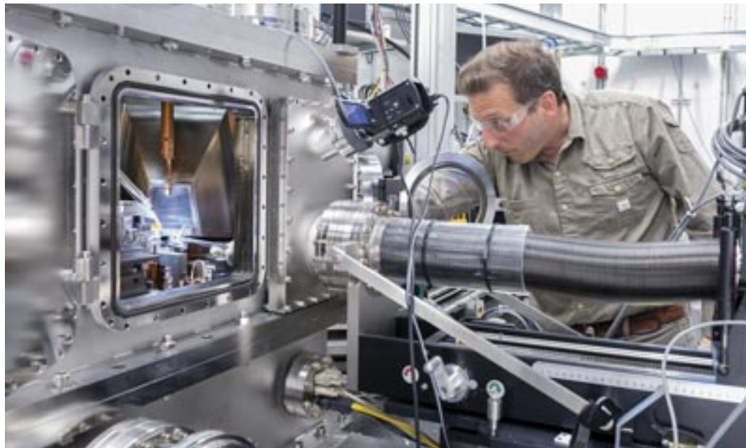
Placing a sample in the Hard X-ray Nanoprobe operated by the CNM and XSD at Sector 26 of the APS. This instrument is used for imaging strain fields near defects and interfaces to understand structural correlations with chemical activity and dynamics in quantum and nanoscale materials for energy.
